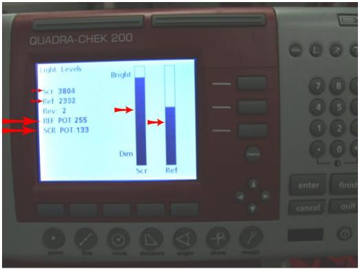
Make sure the "Ref" reading is about ½ to 2/3 of the "Scr" level, and the "Ref" level is lower than the "Scr" level. If not, the cables are in the wrong spot. Check and see that the "Ref Pot" is 255, and the "Scr Pot" is 133. If not, make your adjustments in the lamphouse by the profile lamp to correct it. Make sure the F/O end does not touch the lamp heat shield. Hit "Finish" once.
