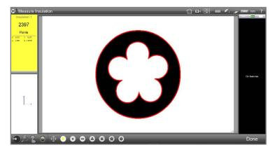
4 Press the Done button to complete the measurement. The insulation will be shown in the Part View and entered into the Feature List.
