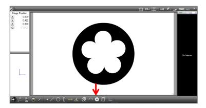
Press or click the insulation edge. The Insulation tool will probe points on the insulation and calculate the shortest and longest distance.
