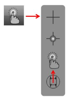
Click the insulation module button in the System toolbar. The button will be displayed at the bottom of the screen. The default method of automatic shape recognition will be enabled.
