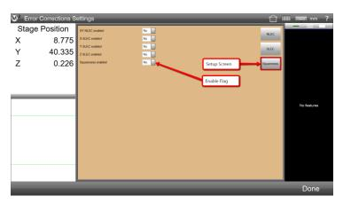
Squareness calibration and correction does not require a machine zero. It is assumed that the angle between the X and Y axis is the same regardless of the current position. A length artifact is used for the calibration, but the actual length does not need to be known. It is only necessary that the length is able to be measured when placed on the stage at a 45 degree angle and at 135 degrees.
