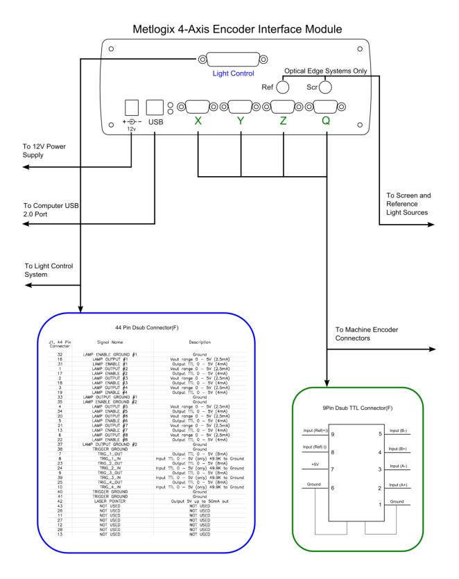
The Metlogix USB Encoder Interface hardware is required to interface encoders to a system running an M3 software package. The following driver installation procedure must be performed prior to achieving successful communication with the Metlogix USB Encoder Interface Hardware.
