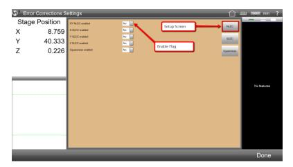
The correction data file is named NlecNew.txt and is located in the settings directory within the Metlogix file output directory. This file is encrypted and may not be changed manually. In a new system, the file is a placeholder only, and will be overwritten when the calibration is performed. The presence of the file does not necessarily indicate the stage has been calibrated.
