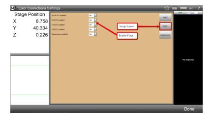
For the original calibration, be sure to disable the SLEC correction under the corrections setup page. It is possible to recalibrate later on using corrected data. That is called an incremental calibration. See comments in step 5 below.
