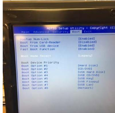
1. Turn off the PC then turn it back on. When this screen is displayed, start hitting the “Delete” Key
