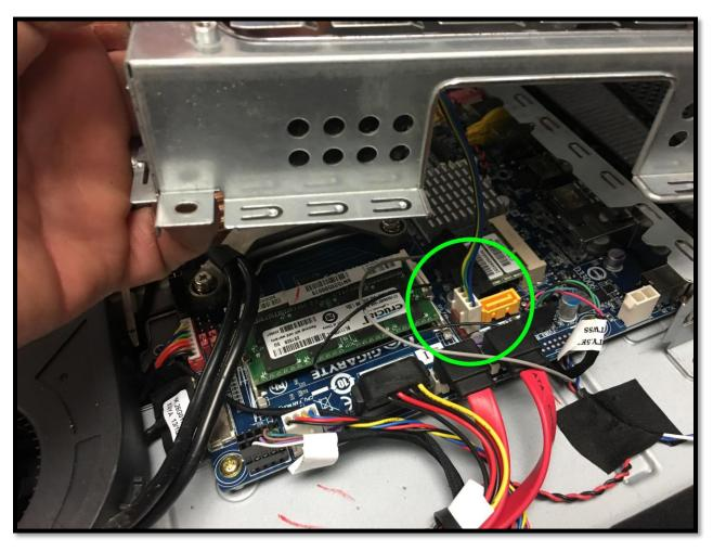
7. Once the shield has been completely removed unplug the SATA power cable from the motherboard and the hard drive. Untwist the cable ties holding the cables in place and remove.
