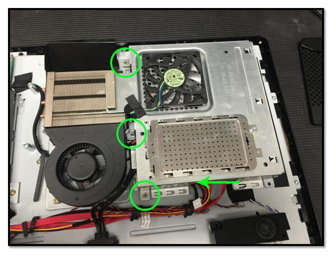
6. After sliding the shield off unplug the fan cable underneath the cover.
