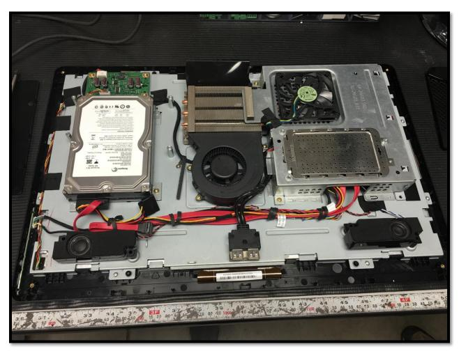
Once the back cover is off remove the three screws hold the RF shield on.
